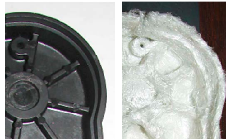
Ashing-Test of LFT-Part
